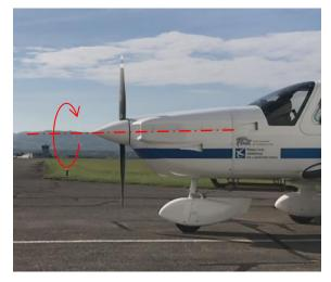
The static rotation test should be carried out over the entire rotation range of the engine. For the first time, make an evaluation during the engine rotation.
