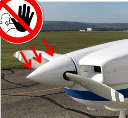
**Moreover, it is forbidden to move the aircraft by handling the spinner or to push on it (leaning on the spinner...)**
