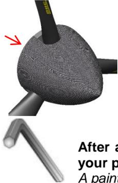
Once all the settings of the propeller were made, mount the spinner of the propeller by tightening the screws to **4Nm (0.4 kg/m; 35lbs/in)** with the appropriate tools.
