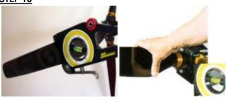
Adjust the pitch angle of the blades with the adjusting tool. See the item 4.4. Adjusting the blade angle of the propeller.
