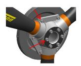
Slightly loosen the screws so that each blade can rotate in its compartment.
