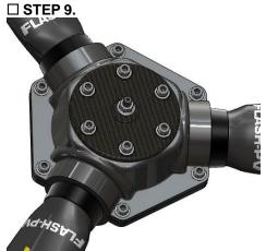
Put the 6 Fixation screws CHC M8 + Washer in the fixations drillings of the propeller.
