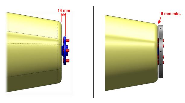
In this case, the hydraulic variable pitch propeller hub is suitable for this type of mounting:
