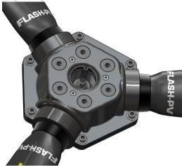
Place the Screws CHC M8x30 + Washer over the top and the Nylstop nut behind for the assembly of the 2 halfhubs.
