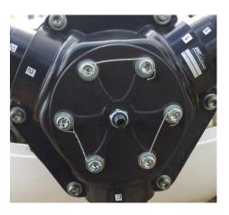
10) After a final check (position and orientation of parts, tightening, ...), install the spinner on the spinner mounting plate by **tightening the screws to a torque of 4 Nm (0.4kg / m)** with the appropriate tools.
