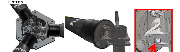
While keeping the satellite laid on the back half-hub, slot the FLASHBLACK/-2 & SWIRLBLACK-3 blades one after the others into the satellite groove and into the back half-hub.
