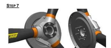
From the back, position the spinner mounting plate according the screws.
