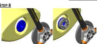
Install the stacked whole on the propeller-shaft (or on the corresponding adaptor spacer corresponding). Tighten moderately.
